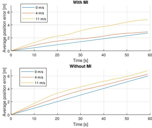
Fig. 6. The mean DR error of the LSTM method for all wind directions at wind velocities of 0, 4 and 11  $\text{m s}^{-1}$ . Top plot: a subset of the elements in the complete input vector was extracted using MI and used as input to the LSTM model. Bottom plot: all entries in the complete input vector was used as input to the LSTM model.
