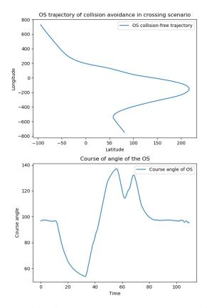
Fig. 8: Collision-free trajectory and the course angle of the OS.
