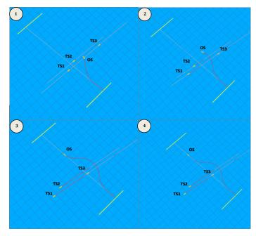
Fig. 7: Simulation result of multi-ship collision avoidance of crossing scenario.
